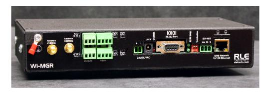
Thank you for purchasing a Wi-MGR wireless sensor network manager. This guide outlines basic installation and configuration. Additional support information, including the User Guide, is available on our website - www.rletech.com. Before you install and configure your device, check the website to ensure you are using the most recent version of our documentaiton.
