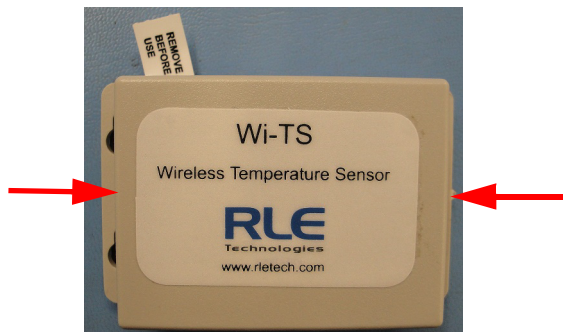
Figure 2.11 Remove the Sensor's Lid
