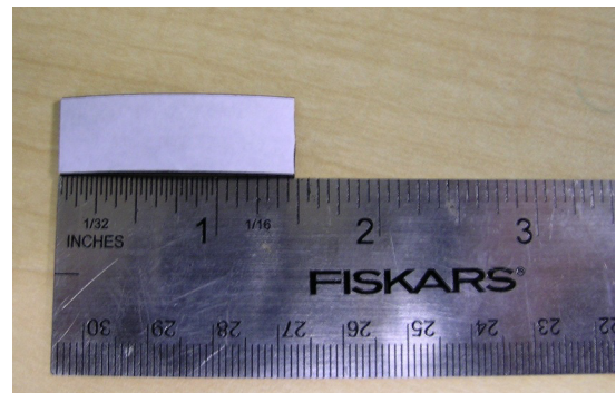
Figure 2.17 Recommended Length of 0.5 Inch for Magnetic Strip
