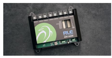
Thank you for purchasing a BMS-1WIRE temperature and humidity monitoring device designed to integrate directly into a building management system (BMS). This guide outlines basic BMS-1WIRE installation and configuration. Before you install a BMS-1WIRE, check RLE's website to ensure you are using the most recent version of our documentation.
